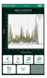
"As part of the 6 second CAT6A++ Autotest, TestPro will perform all standard measurements in addition to extra parameters such as DC Resistance Unbalance, ELTCTL, TCL, fault location, and more for both Channel and Permanent Link."
