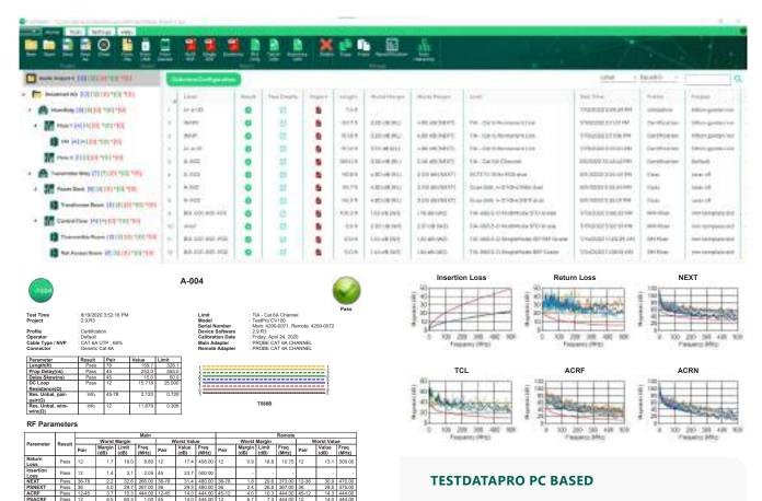
TestDataPro supports both PC and cloud-based options, and is included with all models of TestPro. Printed test reports for copper and fiber optic include a listed of compliant network support based on the performance of the cable tested.
